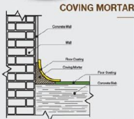
Coving Mortar & Coating System
